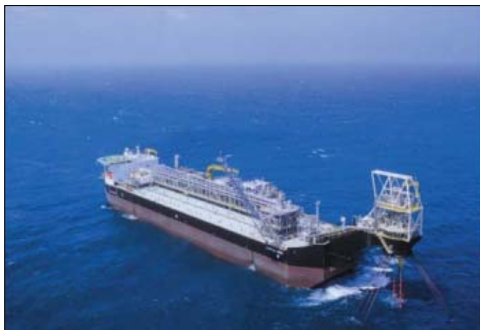
FPSO Cuu Long MV-9 is a double-sided SuezMax class tanker equipped with an external turret (Fig. 5).
